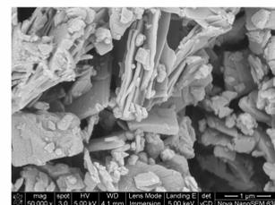
HR-SEM: 85 % in between 1-100 nm (Ø 69 nm plate-thickness) => nanomaterial.
