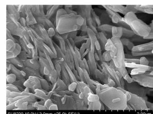
HR-SEM: 33 % in between 1-100 nm (Ø 128 nm plate-thickness) => conventional material.
